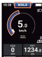
Walk assist mode (assistance functioning)
